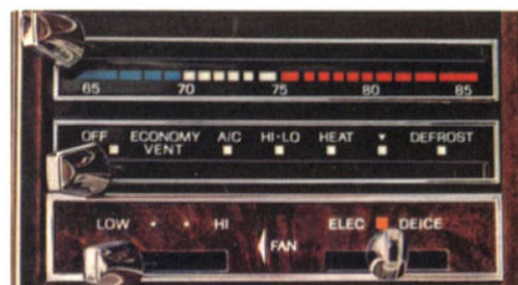
Automatic Temperature Control air conditioning with driver controlled fan speed.
