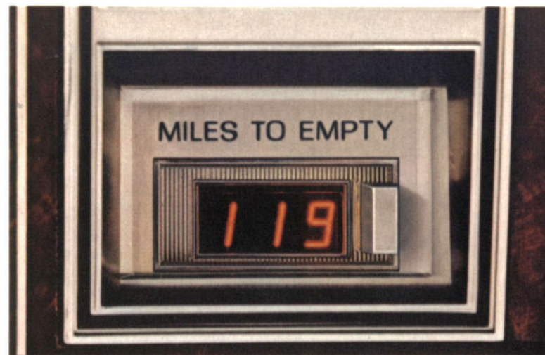
"Miles-To-Empty" Gauge. Standard on Diamond Jubilee Editions, optional on all other Continental Mark V's.
