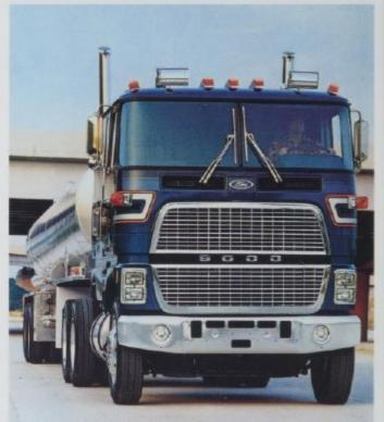
The CLT-9000 all-welded cab is built of high-strength, lightweight aluminium alloy combining toughness with tightness and a quiet ride.
