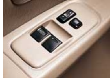
On the Driver Door Armrest, You Will Find Controls for Power Windows and Door Locks (Optional on CE)
