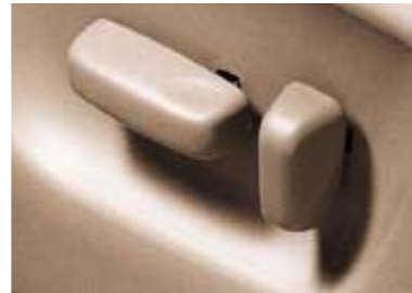
LE's Optional Power Driver Seat Includes Adjustments for Fore & Aft Slide, Seat Cushion Height & Seatback Recline
