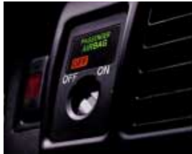
Tacoma's New Driver Controlled Passenger Side Airbag Deactivation Switch Provides Protection for Infants in a Rear Facing Child Seat
