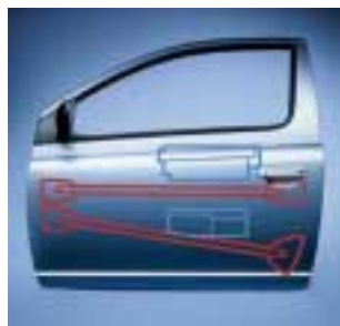
Above: Side-impact door beams made of high-strength steel offer additional protection.
