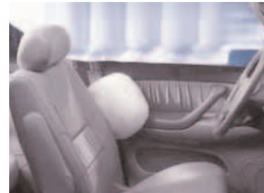
Above: Side curtain airbag system and front seat mounted side-impact airbags (SRS)* Head injuries are one of the most dangerous results of side-impact accidents. The Sequoia is among the very first SUVs to feature side-impact head protection, in the form of side curtain airbags. In the event of a severe side-impact collision, two airbags, located in the overhead roof rail and the side of the front seats, deploy instantaneously, helping protect the driver and front passenger.
