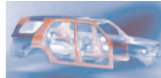
Above top: Specially engineered crumple zones, reinforced A, B and C pillar structures and side-impact door beams.
