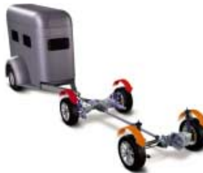
If you carry heavy loads, the rear wheels receive more power to maximize driving stability.
