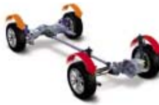
If the front wheels show any tendency to spin, the AWD system responds instantly by redistributing power for maximum stability.
