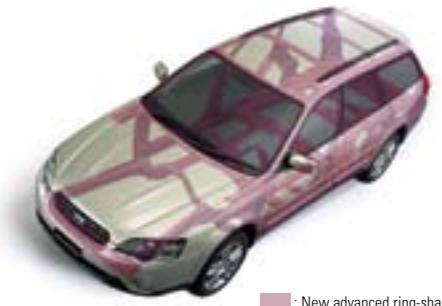
■ : New advanced ring-shaped reinforcement frame
