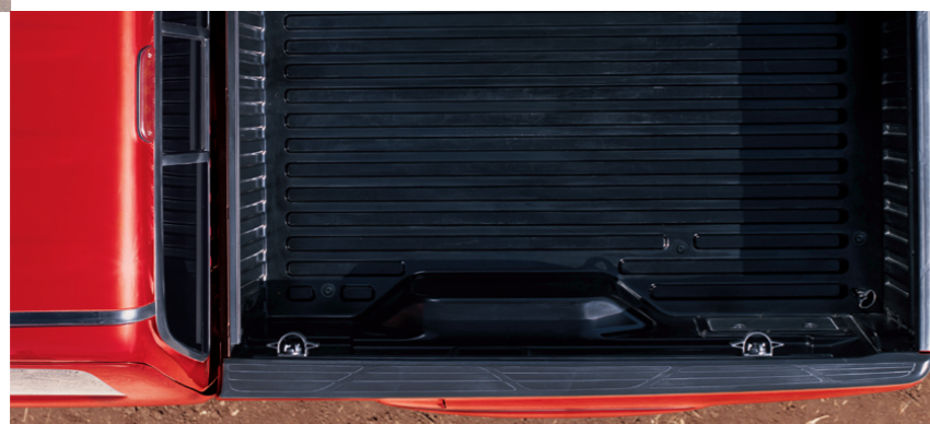
Above top: Tacoma 4x4 Access Cab shown in Radiant Red. Above: Tacoma's 18 inch deep box with the amazing fiber-reinforced sheet-moulded composite bed that has better impact-strength than steel.
