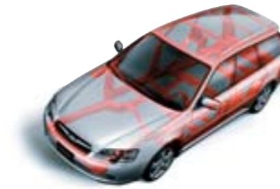
■ : Advanced ring-shaped reinforcement frame
