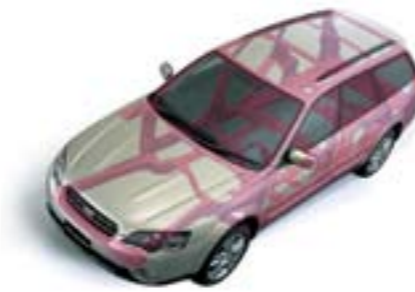
■ : Advanced ring-shaped reinforcement frame
