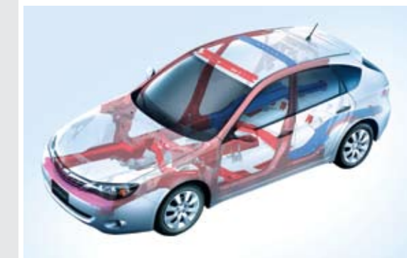
Advanced ring-shaped reinforcement frame
