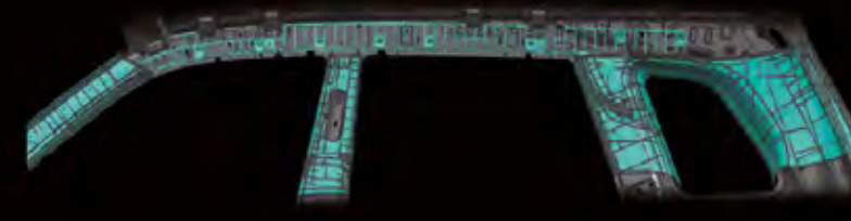
Head-impact protection is built into all pillars and upper cabin surfaces to help minimize head injuries in the event of an accident.
