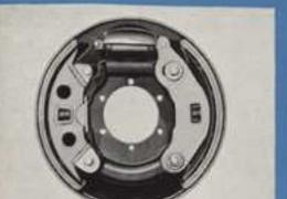
RPAKES—Internal Espanding Hydrawlis Dual Primary type brokes represents note worthy advancement in broking. Hydrovac boaster is aptional.
