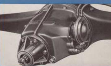
TWO-SPEED AXLE—For the heavier houling jobs, Mosh trucks can be equipped at extra cost with the Timben Two-Speed Double Raduction Hypaid Rose Axle.
