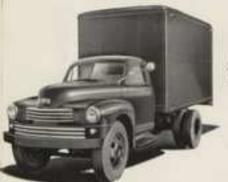
VAN BODY-A 12-foot body of sturdy construction mounted on the 157-inch wheelbase Nash Truck Chassis. Available in both shulght frame and wheelhousing type, in many combinations of side and rear door and tall aste. amengements.
