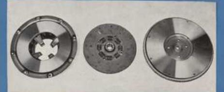
CLUTCH—The loop-life clutch is a single plate 15-inch diameter unit having a reserve of torque capacity to most all operating conditions in heavy tracking.
