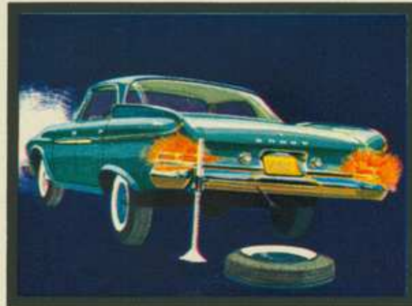
Safety blinkers —when emergency forces you to stop on street or highway you can flash all four turn-signal lights continuously to warn other cars.
