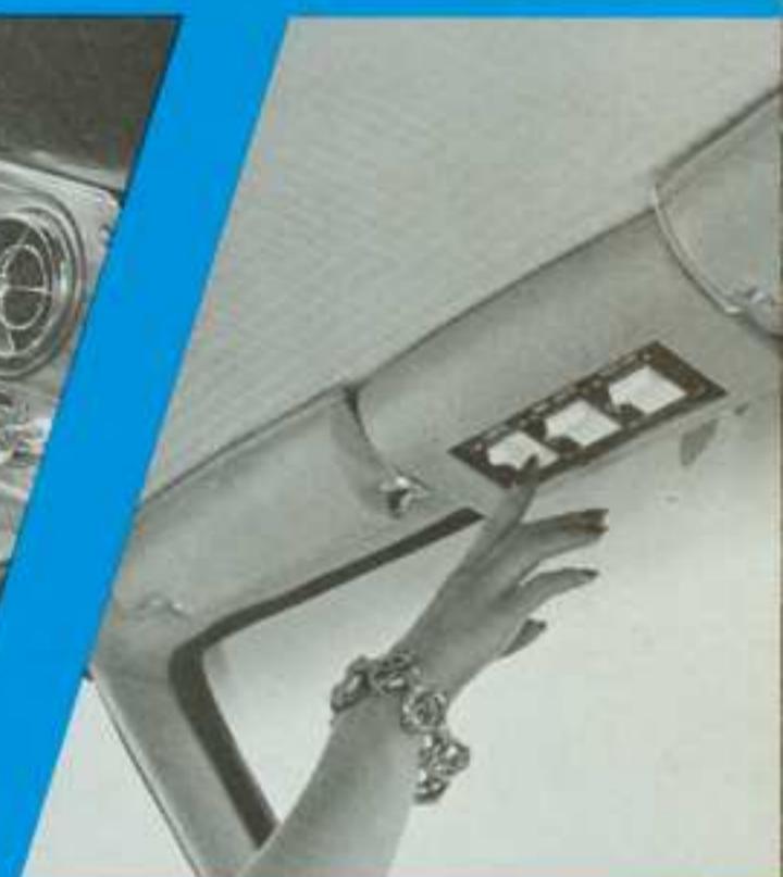
Light switches are overhead for easy access. Lower beam switch on floor operates at a touch of the toe.
