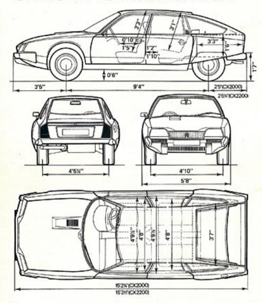
Saloon: 4-door, 5-seater. Max towing weight with standard towing equipment 900 kg, 1984 lbs. Max. fooking weight with additional equipment 1300 kg, 2866 lbs.
