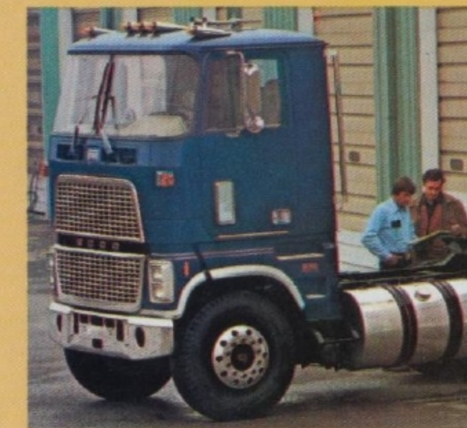
64" BBC. The biggest Ford CL non-sleeper cab, it's available on both single- and tandem-axle chassis.
