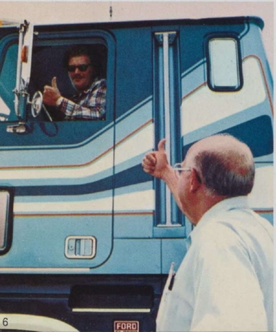
All-aluminum cab. Special wide flanges make panels easy to repair by riveting or welding.
