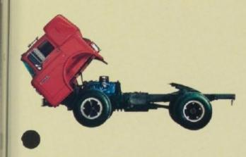
Fresh-air intake supplies cool, dense outside air to the engine for efficient operation. This system is now standard with all C-Series engines. Deep-dip Electrocoat primer helps protect cab against rust and corrosion. Cabs are fully immersed and a high voltage charge bonds primer to the metal, covering areas ordinary sprays can't reach. Step wells
