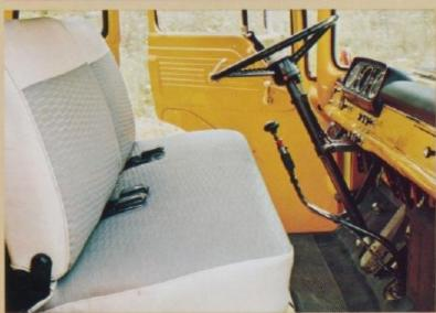
**Standard Cab** on C-600 through C-800 has a foam-padded full-width seat trimmed in gray vinyl. On the C-900, C-800 with 7.8L (475) V-8 and diesels, seat has heavy-duty black vinyl trim (optional C-600 through C-800). Standard features include: pushbutton door locks, reversible key locks, fresh air heater/defroster and removable instrument cluster.
