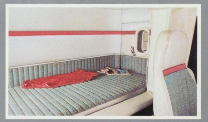
The sleeper compartment is comfortable and carefully appointed with a 6-in.thick innerspring mattress fully 30 in. wide by 80 in. long. Heater, fresh air vents and interior lights are all standard. Built-in radio speakers and controls, dual doors, and mattress cover are included with Custom Hi-Level trim (shown).
