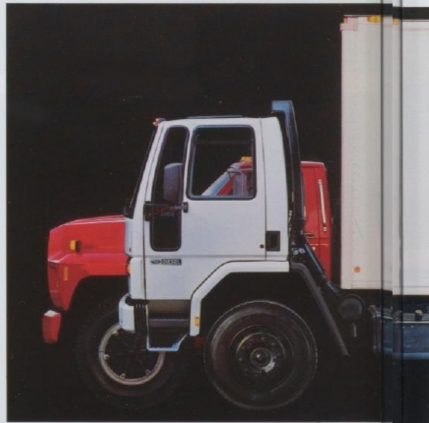
CARGO's shorter overall length (2 feet less than a conventional truck with the same CA) and set-back front axle provide improved maneuverability and better load distribution.
