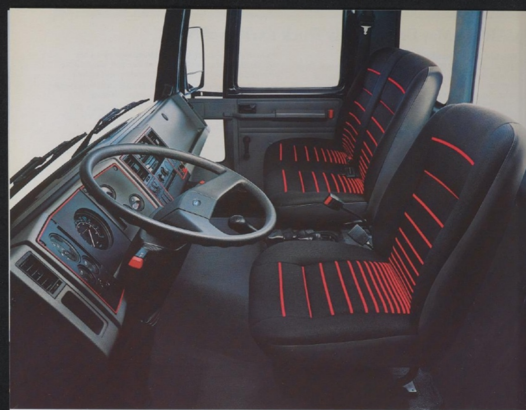
Forward-folding 2-person passenger seat allows easy access to cab storage area.
