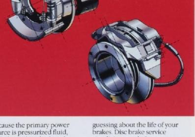
Because the primary power source is pressurized fluid, both the parking brake release and brakes are instantly available at engine start-up. Brake performance is not affected by altitude or rapid number of applications. The booster has an integral electric backup and motor. The motor is automatically actuated to provide braking power if the engine stalls, or if the hydraulic pump flow should drop too low. A brake warning light and buzzer alert the driver in the event of primary pump malfunction.
