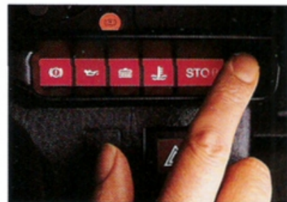
Check button allows verification of all warning function lights.
