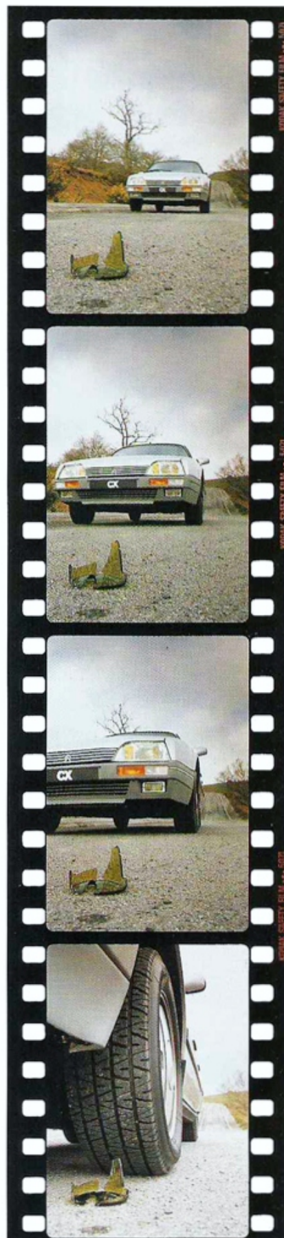
The unique suspension geometry and self-levelling system maintains the CX in a straight line in the event of a blowout.
