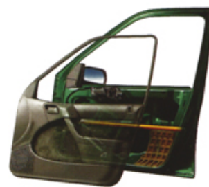
Further protection comes from Xantia's front door energy-absorbing side impact system. In the event of a collision, the panels are designed to deform progressively. This transfers much of the force to the car's structure away from the occupants and helps to reduce the possibility of injury.
