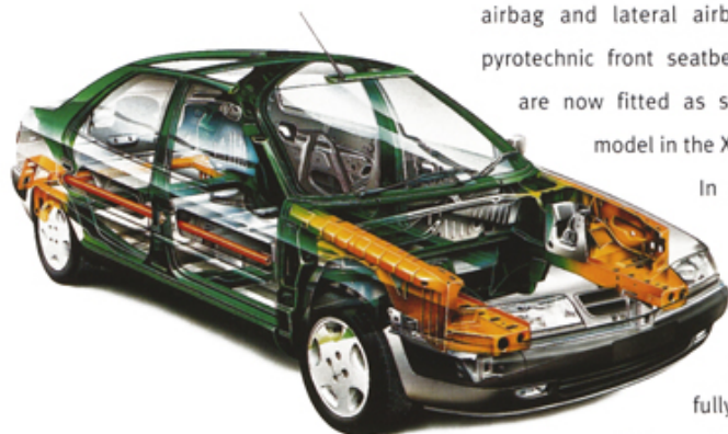
The occupants of a Citroën Xantia sit inside a rigid central cell surrounded by a protective ring of steel and high tensile steel bars in the doors.
