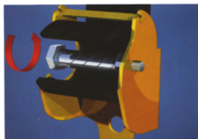
After the action of the pre-tensioners, force limiters in the front seatbelts release slack to reduce the pressure applied to the thorax preventing injury.
