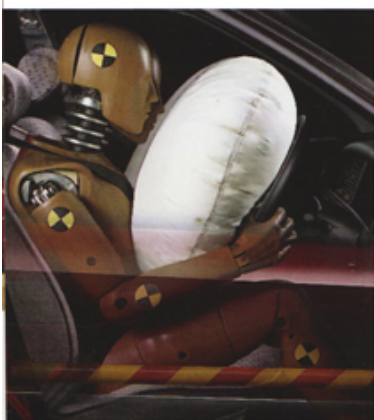
Driver's and front passenger airbags inflate in an accident to protect against injury to head and chest.
