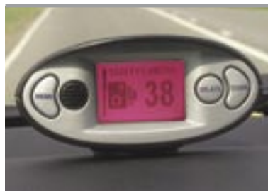
30. The Road Angel Compact (Q82203000) has a simple plug in and go installation and provides visible, spoken and audible alerts of fixed safety cameras and accident black-spots.
