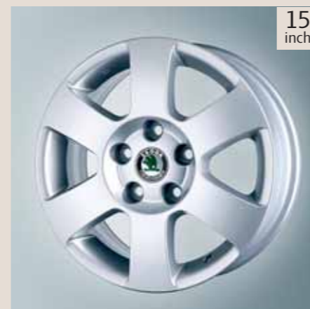
Alloy wheel 6,0J x 15" Orion for tyre 195/65 R15 (CCA 600 003)
