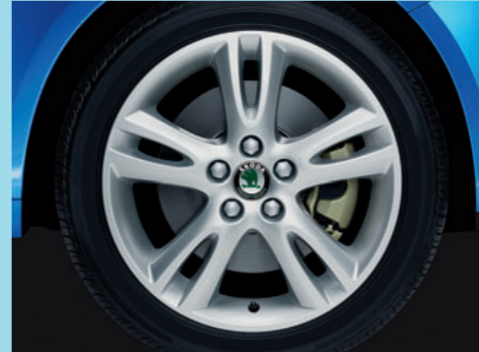
'Atria' alloy wheel 6.5J x16" for tyre 205/45 R16
