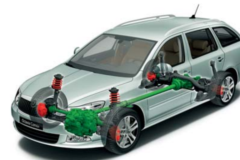
Octavia Combi with a 4-wheel drive and a 4th generation Haldex clutch (1.8 TSI/118kW, 1.6 TDI CR DPF/77kW and 2.0 TDI CR DPF/103kW engines)
