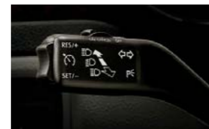
Cruise control for all engine versions for cars with on-board computer (3T0 035 623); for cars without on-board computer (3T0 035 623A)
