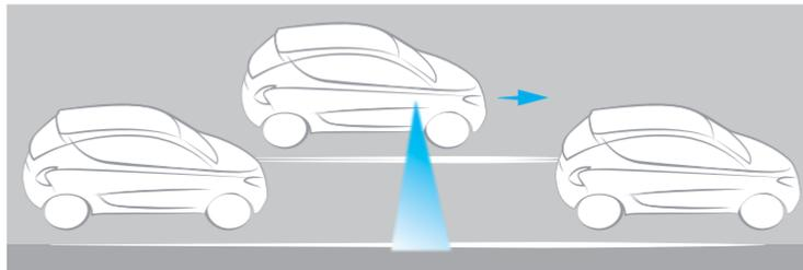
The semi-assisted parking system enables you to find a parking space big enough for your car then helps you park by acting automatically on the steering.
