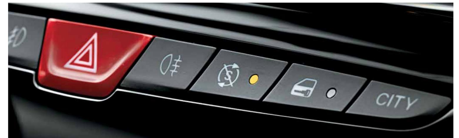
The device can be de-activated when necessary by using the conveniently located dashboard button. There is also a Gear Shift Indicator (GSI) that helps you find the optimum time to change gear, and save fuel.
