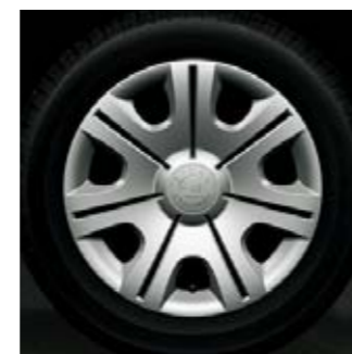
6.0J x 14" steel wheels for 185/60 R14 tyres with Tethys hub covers.
