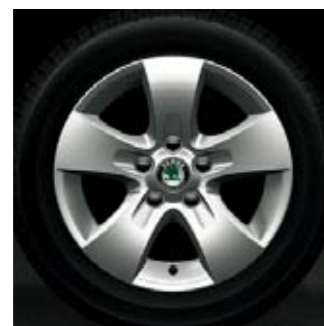
6.0J x 14" Atik alloy wheels for 185/60 R14 tyres.
