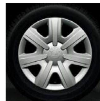
5.0J x 14" steel wheels for 165/70 R14 tyres with Comoros hub covers.
