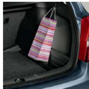
You may hang your shopping bags on folding hooks available on both sides of the luggage compartment.
