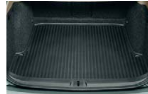
Plastic boot dish with ALU partition; raised 10cm edge (1Z0 061 162) ALU partition can be set in different positions to divide the boot dish storage area Extra ALU partition (3T0 017 254)
