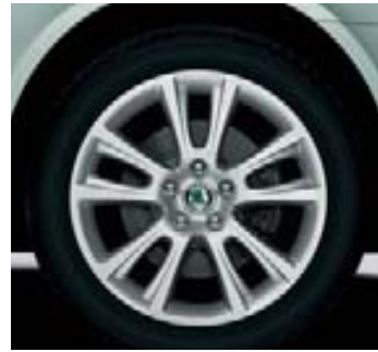
Alloy wheel 7.0J x 17" Zenith for tyre 225/45 R17 (CCH 600 008); 7.5J x 18" Zenith for tyre 225/40 R18; only for RS (CCH 600 009)
