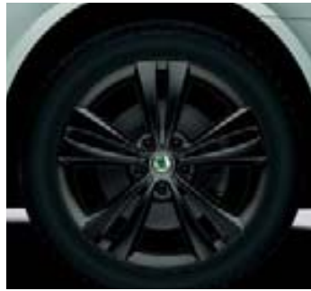
Alloy wheel 7.5J x 18" Neptune for tyre 225/40 R18 in black design; only for RS (1Z0 071 498A)
