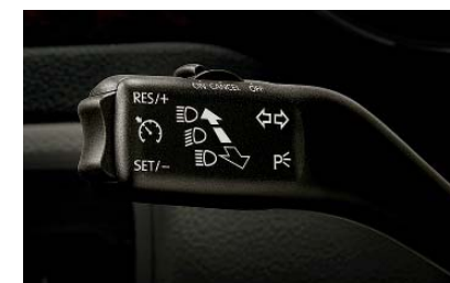
Cruise control for all engine versions for cars with on-board computer (3T0 035 623); for cars without on-board computer (3T0 035 623A)
