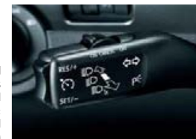
Cruise control for all engine versions for cars with on-board computer (3T0 035 623); for cars without on-board computer (3T0 035 623A)
