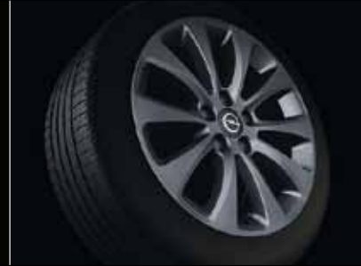
▲ Alloy wheel, 6.5 J x 16, 10-spoke design in Titan finish, tyres 205/55 R 16
