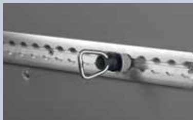
Movable lashing eyes. Purpose designed for the Opel Movano rail system. Made of steel with push-button locking mechanism.
