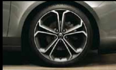
Alloy wheel, 8J x 19", 5-spoke bi-colour design, tyres 235/40 R19 (PZT 5 ).
