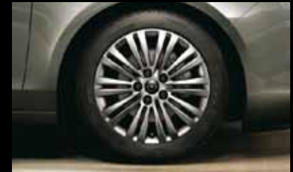
Alloy wheel, 7J x 17", 10-twin-spoke design, tyres 225/50 R17 (PXS 4 ).
