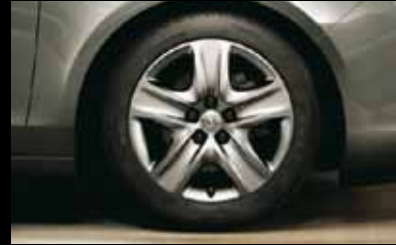
Structure wheel, 7J x 17", 5-spoke design, tyres 225/50 R17 (PWT 1,5 ).
