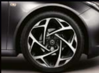
12 Alloy wheel, 8.5 J x 19, 6-Y-spoke design, tyres 245/40 R19 (Q7P).
