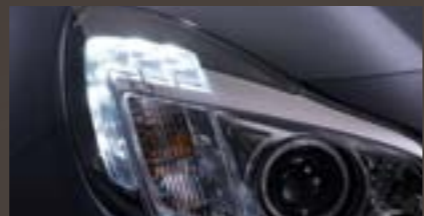
LED Daytime Running Light. Attracts the attention of other road users without increasing fuel consumption (unlike low beam).
