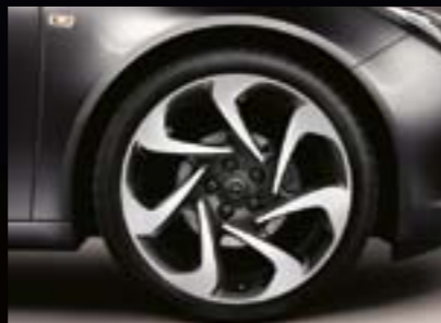
13 Alloy wheel, 8.5 J x 20, 7-wing-spoke design, tyres 245/35 R20 (Q7R).
