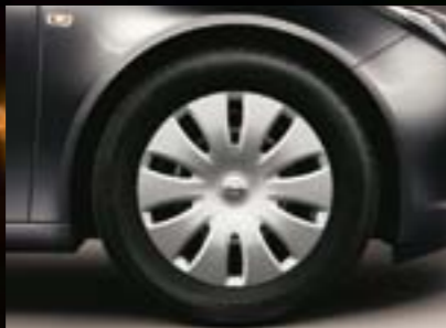
2 Steel wheel incl. cover, 7 J x 17, 10-spoke design, tyres 225/55 R17 (QR4).
