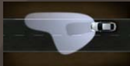
Adverse Weather Light (up to 70 km/h). Wiper or rain sensor activated for better vision in bad weather conditions.
