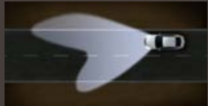
Country Road Light (55–115 km/h). Wider spread and brighter light than normal low beam. 70 metre range without dazzle.
