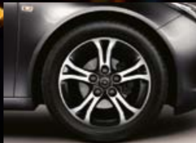
8 Alloy wheel, 8 J x 18, 5-twin-spoke design, tyres 245/45 R18 (Q7B).
