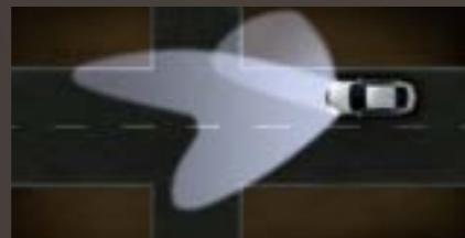
Static Cornering Light (up to 40 km/h, also when reversing). Throws light 90 degrees left or right for enhanced lateral vision.
