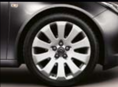
11 Alloy wheel, 8.5 J x 19, 10-spoke design, tyres 245/40 R19 (Q9S). Cast alloy with machined bright finish.
