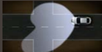
Town Light (30–55 km/h). Wider and lower spread of light. Activated by vehicle speed together with street lighting.
