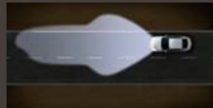
Highway Light (over 115 km/h). 140 metre range, higher and brighter than normal low beam, without dazzle.
