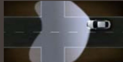
Pedestrian Area Light (up to 30 km/h). Wider spread of light (an extra 8 degrees left and right) illuminates potential hazards.
