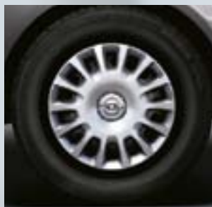
Steel wheel incl. cover, 5.5 J x 14, 14-spoke design, tyres 185/70 R 14
