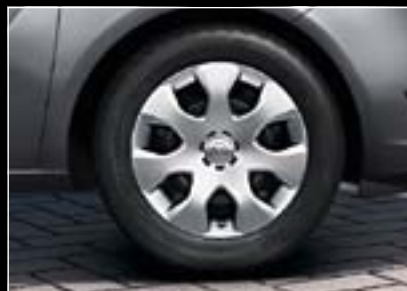
Steel wheel incl. cover, 6,5 J x 15", 7-spoke design, tyres 195/65 R 15 (PA7). 1 Or 6,5 J x 16", tyres 205/55 R 16 (PY3). 2
