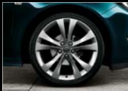
Alloy wheel, 8,5 J x 20", 5-twin-spoke design, alloy with premium multi-coat painted finish, tyres 245/35 R 20 (RTH). 5,7,8
