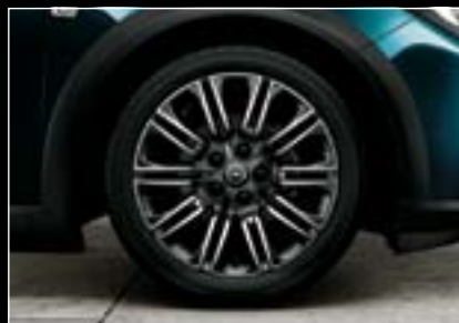
Alloy wheel, 8 J x 18", 10-twin-spoke design, bi-colour finish, tyres 235/50 R 18 (REP). 2
