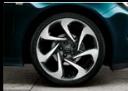
Alloy wheel, 8,5 J x 20", 7-wing-spoke design with bi-colour finish, tyres 245/35 R 20 (Q7R). 5,7,8
