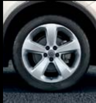
18" 5-spoke alloys in Sterling Silver. 7 J x 18", tyres 215/55 R18. (RV6, standard on drive!, option on Enjoy.)
