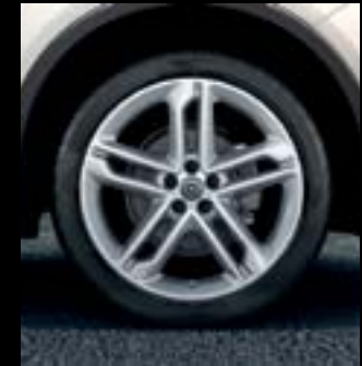
19" 5-spoke alloys in Sterling Silver. 7 J x 19", tyres 225/45 R19. (RT7, option on Enjoy and Cosmo.)
