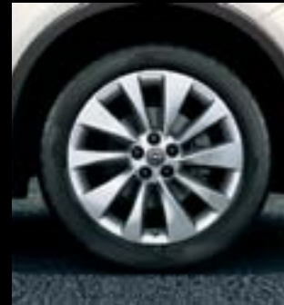
18" 10-spoke alloys in Sterling Silver. 7 J x 18", tyres 215/55 R18. (RV8, standard on Cosmo.)
