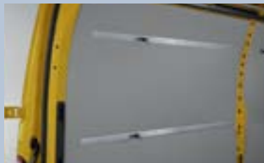
Side anchorage rails. With fixing points every 25 mm, supplied with 6 movable lashing eyes, providing universal load securing.
