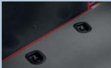
Fixed load lashing eyes. Ideally located, 6, 8, 10, or 12 floor load lashing eyes (depending on vehicle length) keep loads secure and safely in place. 4 side-mounted lashing eyes are also optionally available.
