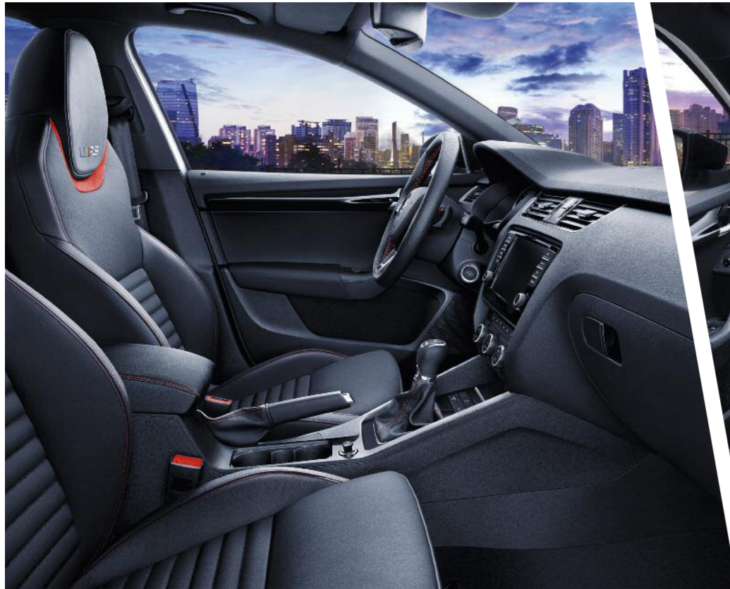
The leather interior is adorned with red stitching and with decorative inserts in black. The electrically-adjustable sports front seats are equipped with memory function and can store three different positions of the seat and the door mirrors.
