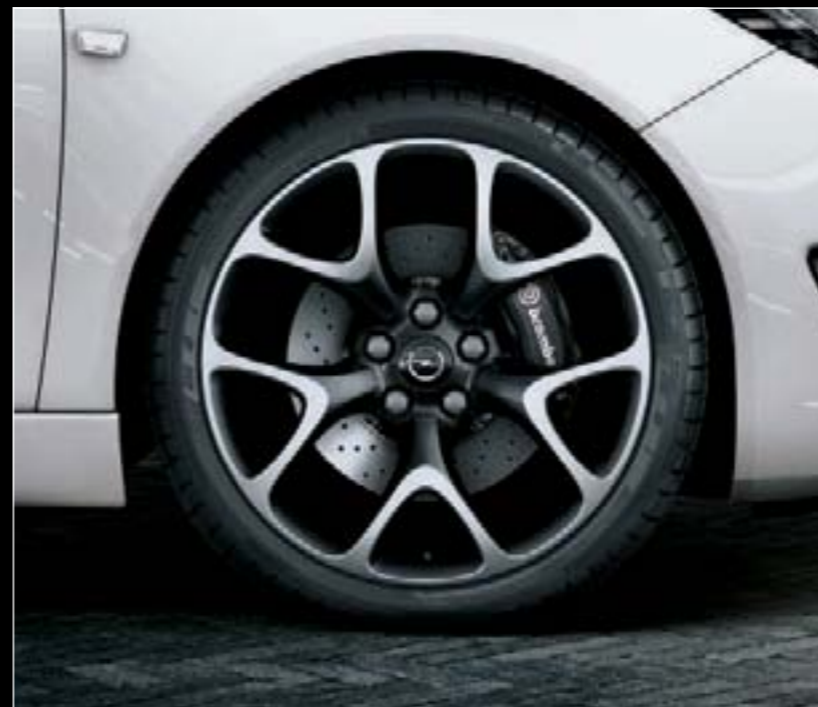
OPC alloy wheel, 8,5 J x 20", 5-Y-spoke design with bi-colour finish, tyres 255/35 R20 (RTJ).
