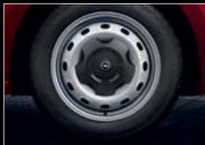
16" steel wheel with centre cap, 6J x 15", tyres 205/65 R 16 (P91).
