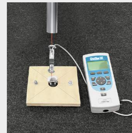
Testing of fixing element strength
