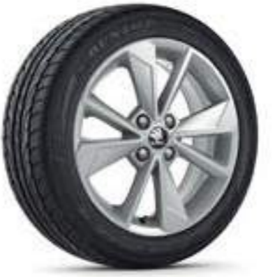
Scorpius 1ST 071 496H 8Z8 Light-alloy wheel 6,0J x 16" for 185/50 R16 tyres in silver metallic design
