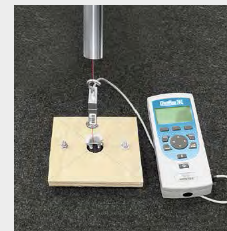
Testing of fixing element strength
