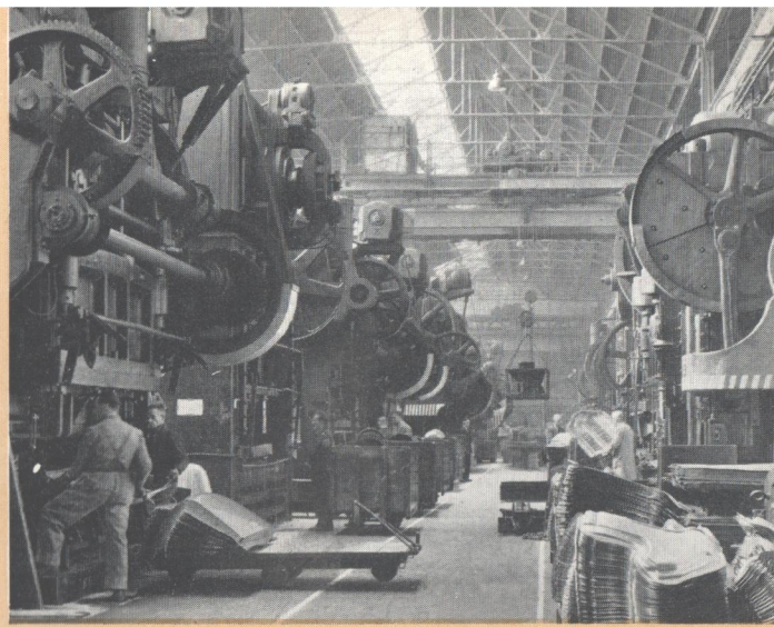
Body panels being shaped by giant machines in the Austin press shop.
